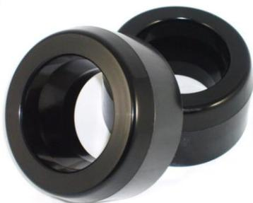
**\*The spacers included in this kit may not represent the actual lift you will achieve with any Performex™ Leveling or Lift kit. Example: A 2.5" Leveling Kit will have 1.25" inch spacers included. Due to independent suspension design on the vehicles, the lift will be approximately double the size of the actual spacer. For any questions please [Contact Us](#) for additional assistance.**
